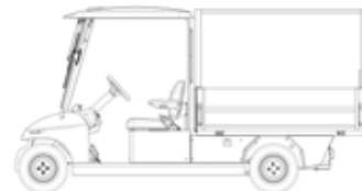
Aluminum Case with Canopy W: 1317 x L: 1800 x H: 1236
