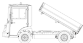
Aluminum Open Frame with Tipper W: 1310 x L: 2240 x H: 440
