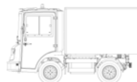
Composite Closed Case with Back Cover W: 1320 x L: 1910 x H: 1200
