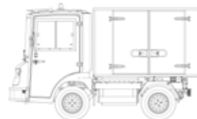
Composite Closed Case with Side Cover W: 1320 x L: 1910 x H: 1200
