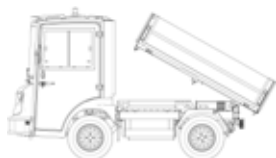
Aluminum Open Frame with Tipper W: 1310 x L: 1910 x H: 440
