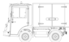
Composite Box Body with Rear and Side Doors W: 1320 x L: 1910 x H: 1200
