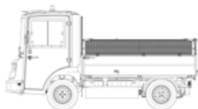
Raised Steel Open Frame W: 1310 x L: 2240 x H: 735
