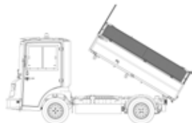
Raised Steel Open Frame with Tipper W: 1310 x L: 2240 x H: 735
