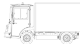
Composite Closed Case with Back Cover W: 1320 x L: 2310 x H: 1350
