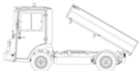
Steel Open Frame with Tipper W: 1310 x L: 2240 x H: 400
